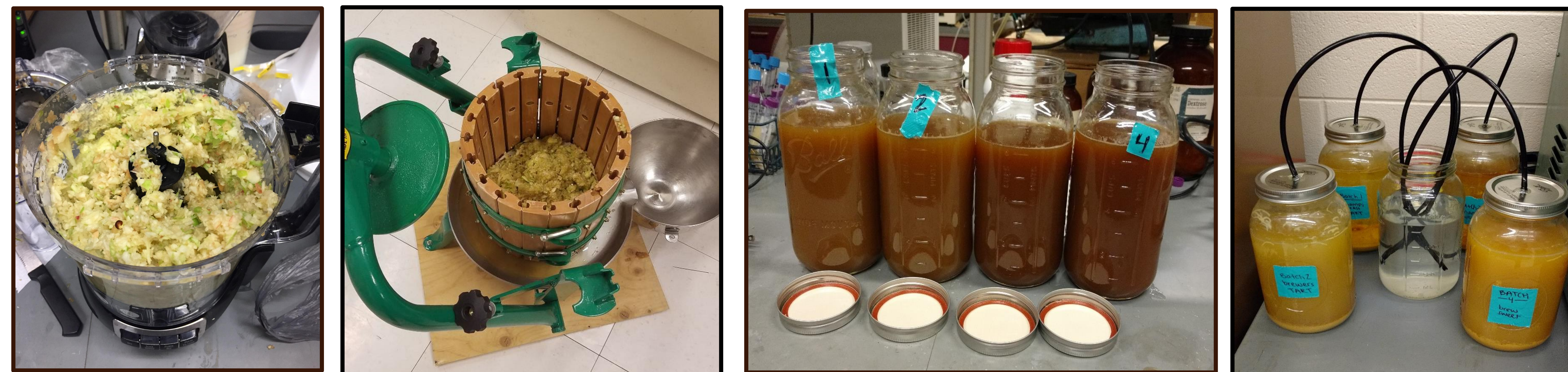
Apples were first "milled" using a food processor and then pressed for juice. The juice was fermented using the self-developed apparatus above. Process variables were determined using a Plackett-Burman design.
